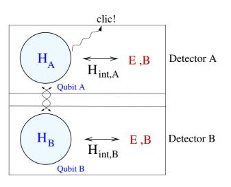
Two 2-level atoms (qubits) initially in state  $|\psi\rangle=\sum_{s,s'=0,1}c_{ss'}|s\rangle|s'\rangle$  are coupled to independent
