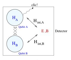
Two 2-level atoms (qubits) initially in state  $|\psi\rangle = \sum_{s,s'=0,1} c_{ss'} |s\rangle |s'\rangle$  are coupled to the **same** modes of the electromagnetic field initially in the vacuum.
