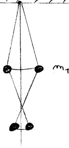
$$\underline{\text{mode 2}} \quad \Omega_2 = \sqrt{2} \Omega_1$$
