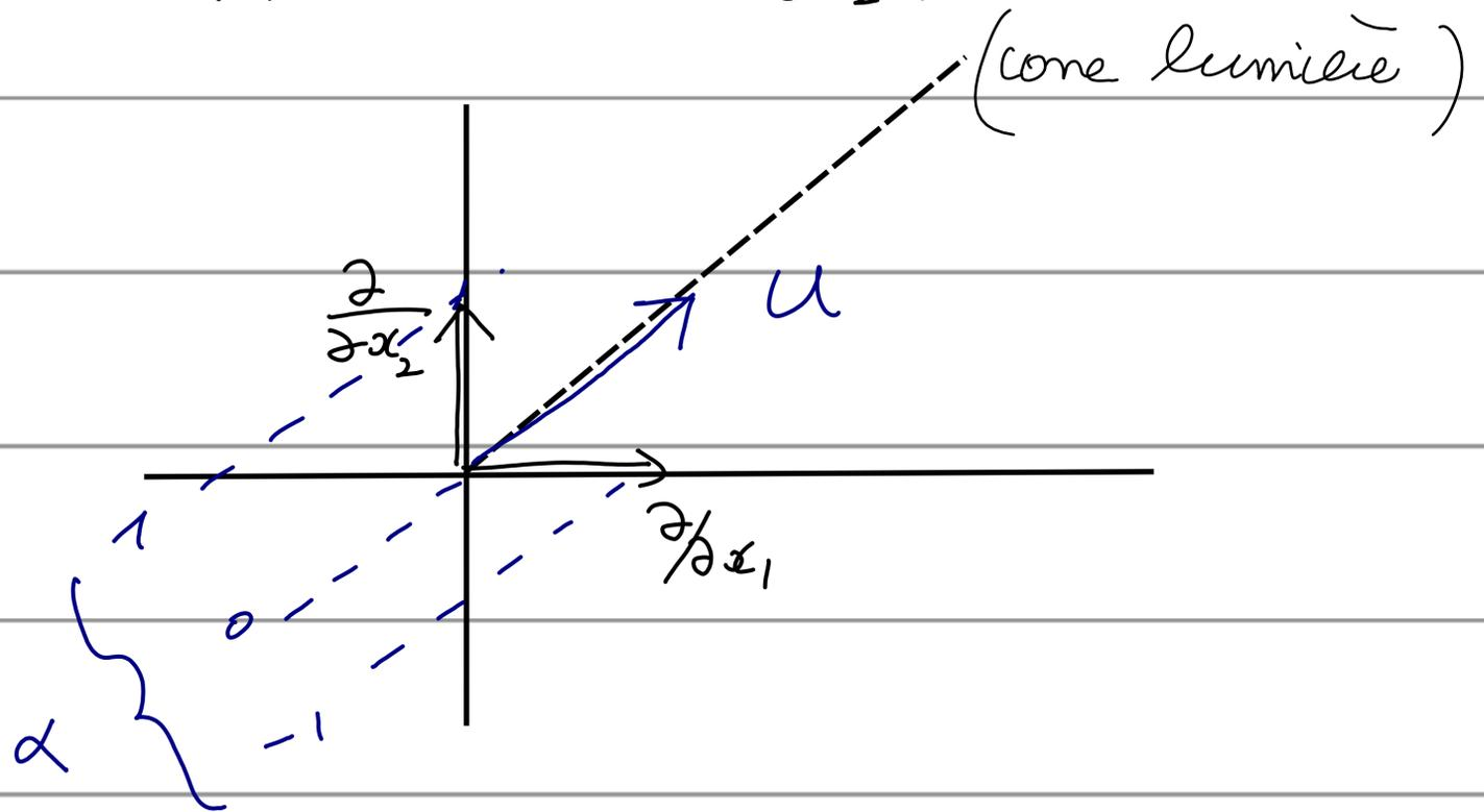
$$U = 2\left(\frac{\partial}{\partial x_1} + \frac{\partial}{\partial x_2}\right), \quad \alpha = \check{g}(U) = -2dx_1 + 2dx_2$$
