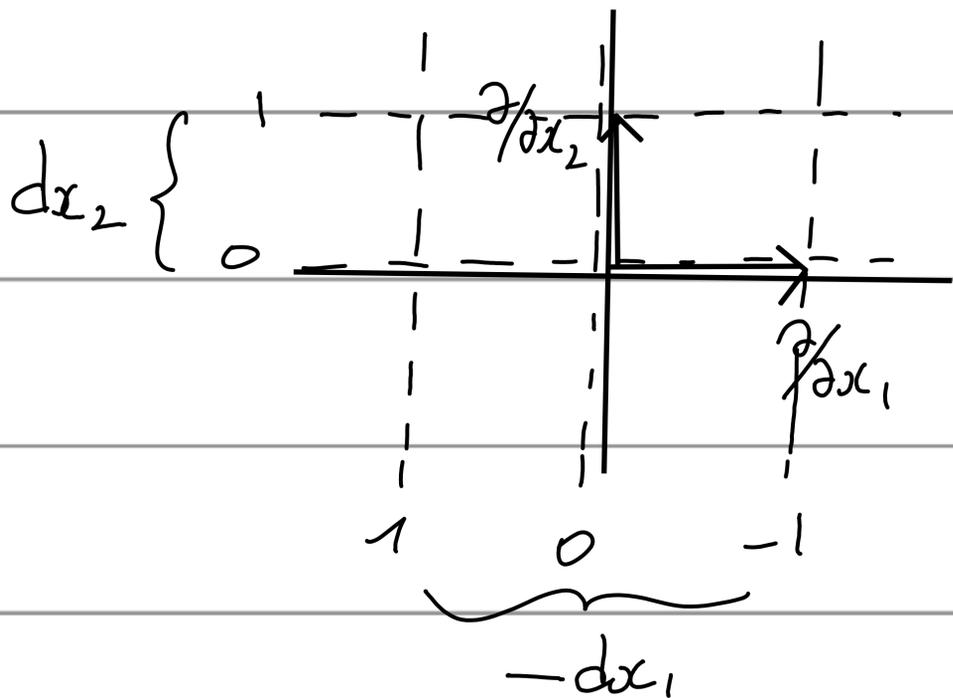
•  $U = 2 \frac{\partial}{\partial x_1} + \frac{\partial}{\partial x_2}$ ,  $\alpha = \check{g}(U) = -2dx_1 + dx_2$
