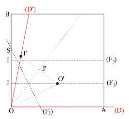
Folding along (F3) so that O is brought to  $O' \in (F_1)$  and I is brought to  $I' \in D'$  constructs the trisection of angle(D, D')!
