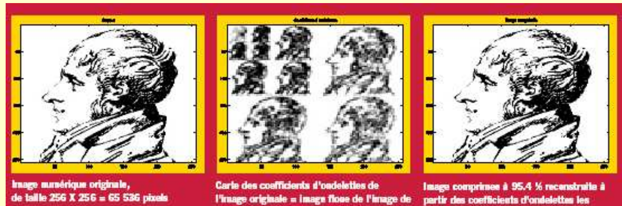
LJK – Fourier's profile compressed @ 95.4% using wavelets
